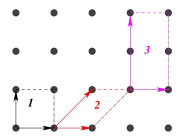
$N_a$ : Number of atoms per unit cell (basis) For unit cells 1 and 2,  $N_a = 2$ . For unit cell 3,  $N_a = 4$ .
