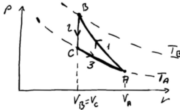
$$L = L_{AB} + L_{BC} + L_{CA} = -\Delta U_{AB} + L_{CA} = nc_V(T_A - T_B) + nRT_A \ln \frac{V_A}{V_C}$$
