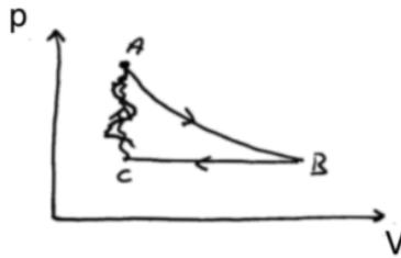
$$Q_{AB} = L_{AB} = nRT_A \ln \frac{V_B}{V_A} = nRT_A \ln 2$$
