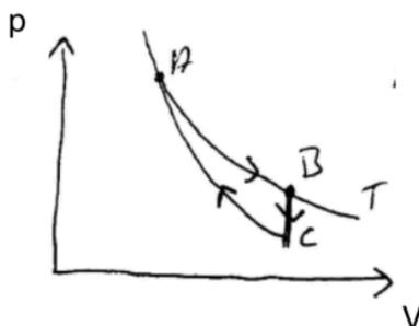
$$\begin{aligned} Q_{tot} &= Q_{AB} + Q_{BC} = L_{AB} + Q_{BC} = \\ &= nRT_A \ln \frac{V_B}{V_A} + nc_V(T_C - T_B) = nRT_A \ln 2 + nc_V(T_C - T_A) \end{aligned}$$
